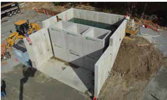
Fig. 3: The dam was assembled from six precast concrete modules. The completed assembly was tested under a constant head in a reinforced concrete tank constructed at the FDE facility in North Billerica, MA
